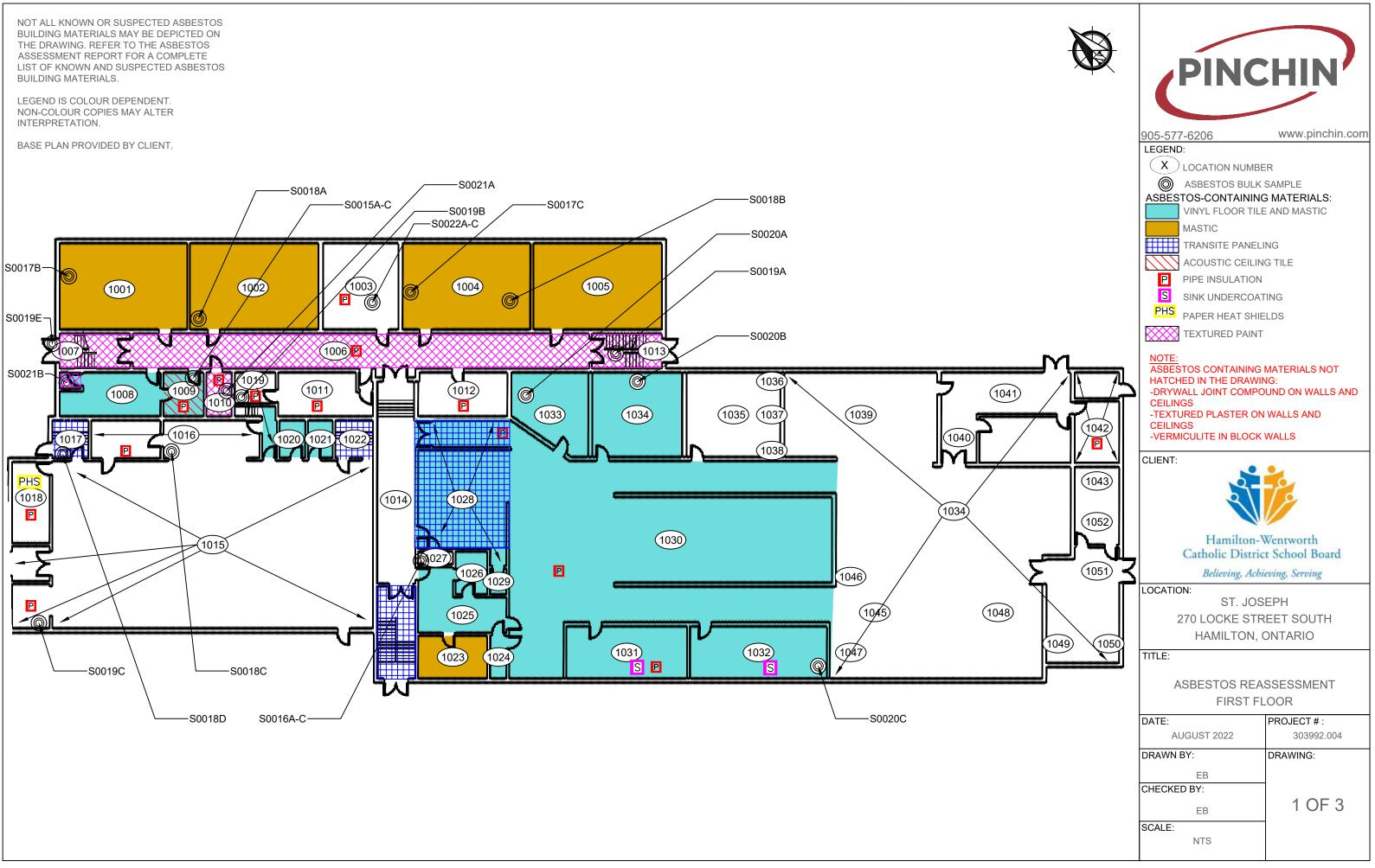
NOT ALL KNOWN OR SUSPECTED ASBESTOS BUILDING MATERIALS MAY BE DEPICTED ON THE DRAWING. REFER TO THE ASBESTOS ASSESSMENT REPORT FOR A COMPLETE LIST OF KNOWN AND SUSPECTED ASBESTOS BUILDING MATERIALS.
